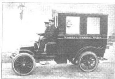
Pneumatic tyres and front-wheel drive are employed; the system is not superior to that of the Metropolitan Asylums Board.
